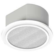
The flame-resistant metal housing has a low installation depth of only 97 mm. Efficient installation on the construction site is possible with the supplied mounting template. A paint cover enables the front grille including the cover to be painted without any problems.
