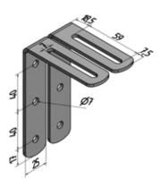
Discreet L-bracket set for extremely close mounting of the speaker to the wall. Side swivel with inclination up to 5°. The speakers housing plates are equipped with M6 inlet threads. Incl. 2x M6x14 hexagon socket screws. Load capacity: 30 kg Dimensions (W x H x D): 20 x 60 x 80 mm
