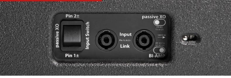
corrections required. A recessed switch on the connection panel enables the signal input to be switched from pin 1 + / 1- to 2 + / 2-. With two monitors wired in daisy chain, two AUX feeds can be played out using normal 4-pin cables without the need for a special interchangeable cable, and the tap can be conveniently set on the monitor. In total four four-pin Speakon NL4 connectors are located on each side and rear of the monitor to enable flexible connectivity.
