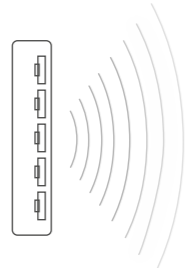
Point source spherical radiation, high volume decrease
