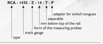
All devices can be delivered from 500 mm nominal gauge upward. The devices are insulated.
