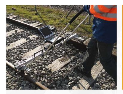
MessReg CTS is an especially efficient and ergonomic measuring system used to inspect geometric track parameters.
