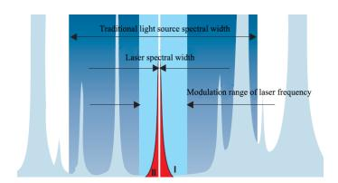
And after obtaining the second harmonics absorbed by detected gas, it finally works out the concentration of detected gas by using this second harmonics and linewidth.
