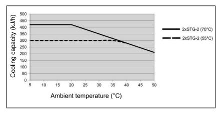
Note: The limit curves of the heat exchangers apply to different dew points, see legend.
