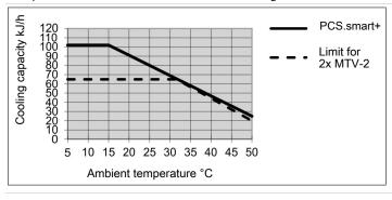
Remark: The limit curve for the heat exchanger applies to a dew point of 50  $^{\circ}\text{C}.$
