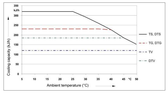
Remark: The limit curves for the heat exchangers exchanger apply to a dew point of 65 °C.
