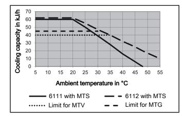
A selected output dew point of 10 or 15  $^\circ C$  shifts the curves 5 or 10  $^\circ C$  to the right.
