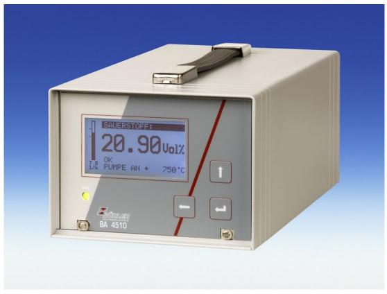
The BA4510 is designed for measurements of oxygen traces in inert gases. It is based on an advanced, zirconia measurement cell. The highly selective cell combines high mechanical strength with consistent accuracy. With inert gases, the cell delivers an increasing signal if the partial pressure of oxygen drops thus giving a highly precise measurement of trace oxygen levels. The value is shown on the digital display and a current output is provided.
