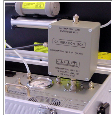
Optional Calibration Box is already set for 1 par Cal. Gas Inlet Pressure
