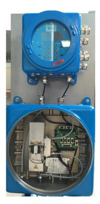
Our innovative photoacoustic spectrometer is based on patented Helmholtz resonance cell combined with Laser Diode, Tunable Diode Laser or Quantum Cascade Laser suitable for trace gas and bulk gas detection.
