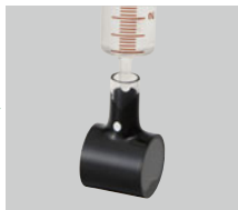
② Inject measuring solvent into cell
