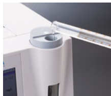
① Inject water sample, solvent
