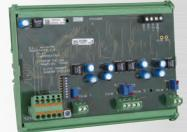
Addressable 4- analogoutput module which delivers 4 analog 4-20mA signal outputs (detector output copy, min, max, average of a group of detectors) for connection to a datalogger, a PLC, a Building Management System (BMS), etc.
