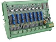
This module enables standard analog transmitters (gas or flame detectors for instance) to be connected on a digital line for cost savings.
