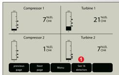
1 Up to 16 detectors can be displayed simultaneously
