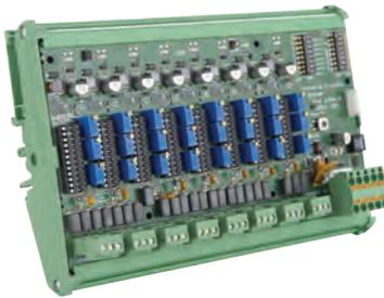
This module enables standard analog transmitters (gas or flame detectors for instance) to be connected on a digital line for cost savings.
