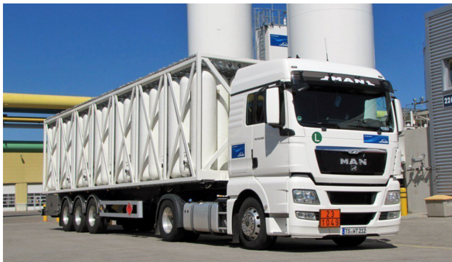
Hydrogen transport with a 500 bar hydrogen trailer. Image: Linde
