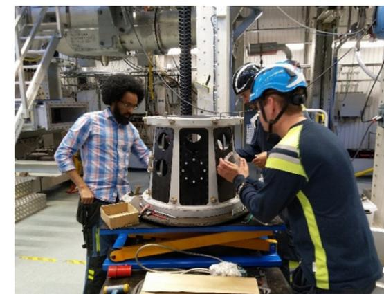
Figure 2. Assembly of the draft tube cone.
