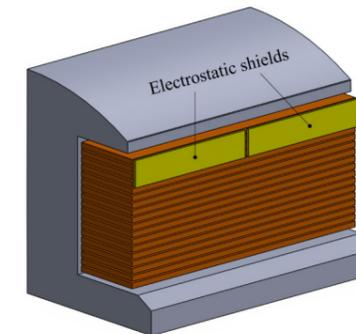
**Figure 2. Pone of the measures for attenuating the high voltage gradient in the field winding.**
