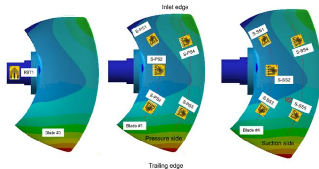
**Figure 4.** Strain gauge sensor locations on the runner blades and the turbine shaft.
