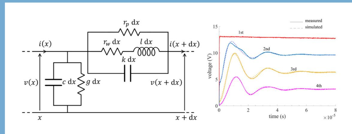
The first part of my work under task 4.2 WP4 of the HydroFlex project has been to determine the parameters of the field winding and of the PE which affect the voltage surges and voltage gradients in the rotor winding of salient pole wound SM. An electric model for reproducing the influence of said parameters has been carried out and tested (Fig.1) together with the experimental setups to be used.
