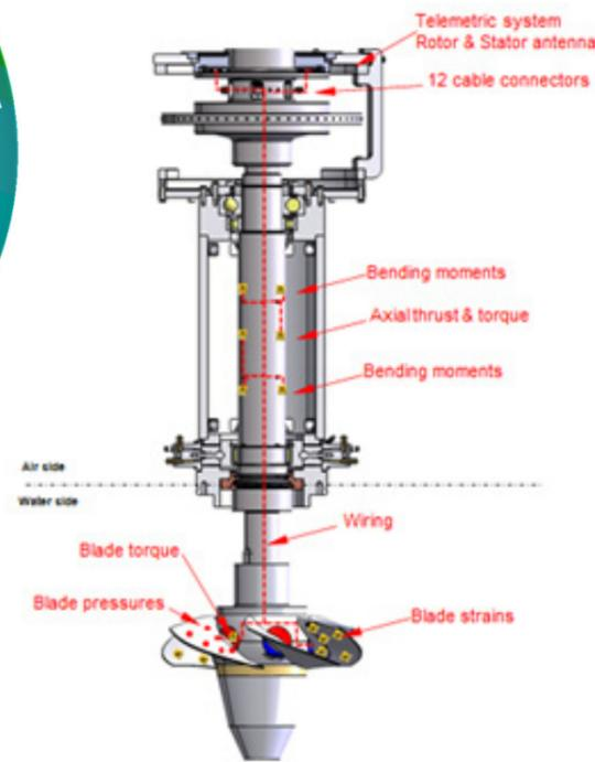
the structural response from excitations originated from the runner, waterways or the AFC4Hydro subsystems (ICM, IPM) will be influenced by its modal characteristics. Depending on the ratio between the excitation frequency and the eigenfrequencies, damping or amplification can occur for the measured quantity.
