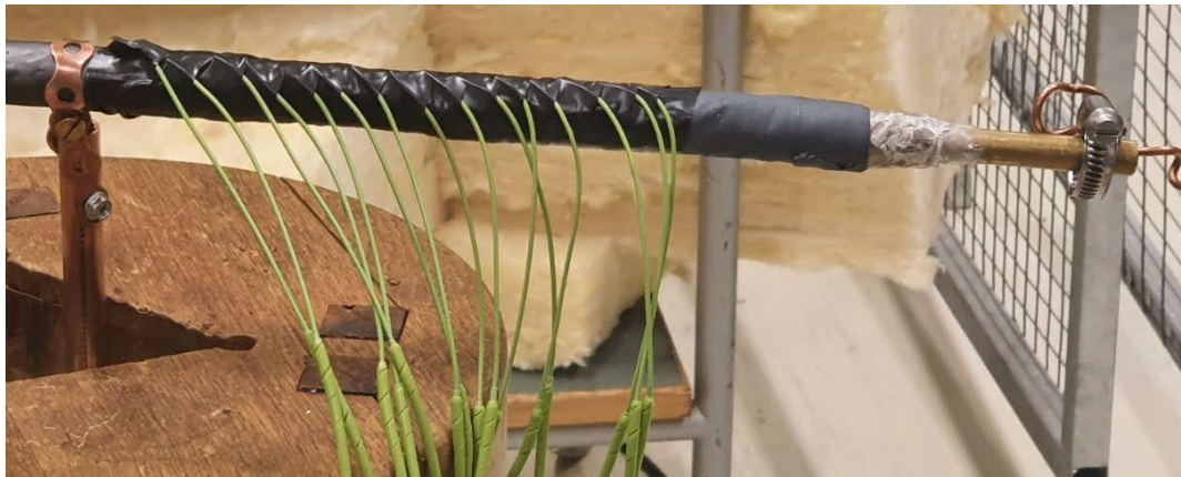
Figure 3-11: Picture of the measurement of surface temperature.
