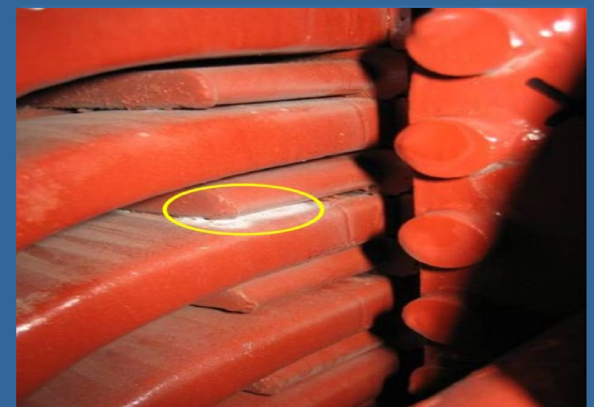
The effect of pressure finger on performance of SG
