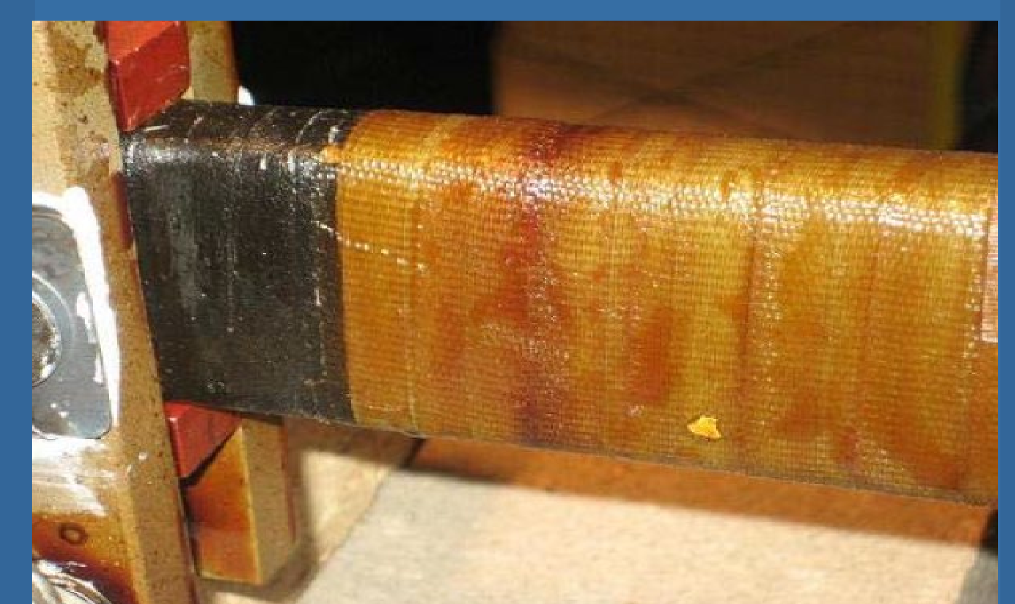
The effect of overlapp methods and resin insulation on SG layer
