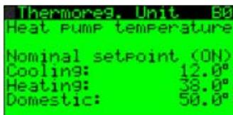
In B01 it can be set the temperature set point of the ON mode:
