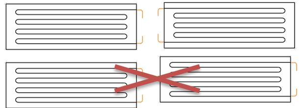
If the panel is installed at horizontal position, it is recommended to install pair of panels confronted for having less piping towards the distributor.
