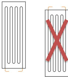
When the panel is installed in vertical position, always the inlet and outlet connection has been at the bottom. (It is not allow to install the reverse)
