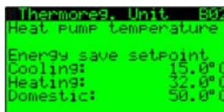
In B2 screen it can be set the temperature set point of Energy Save Mode
