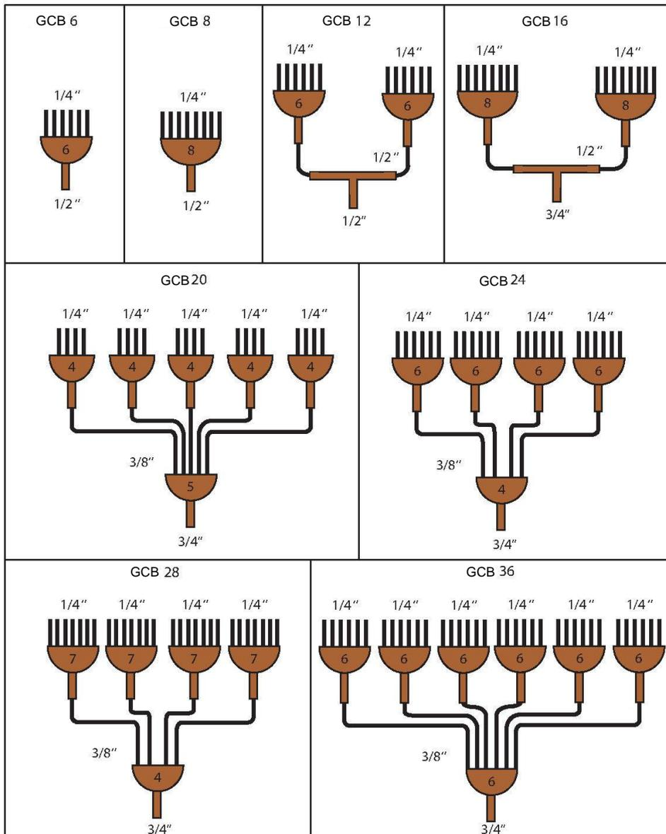
Install the distributor vertically, face upwards according to the picture.
