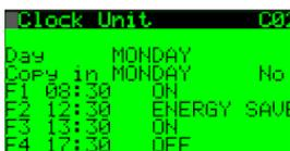
C02: Time bands. Four different can be set on an any day, with the corresponding set point.
