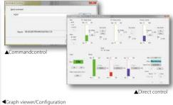
Wavy is an application software that supports sequence creation and the operation for Kikusui power supplies and electronic loads.
