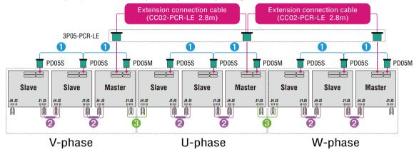
Accessories for three-phase driver and parallel operation driver 1 Connecting cable (0.7m) 2 Power signal cable (0.3m) 3 Power-sync cable (Accessories 1m) \*equivalent to the LC01-PCR-LE
