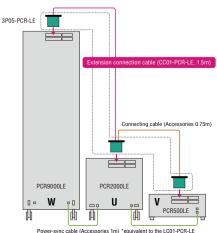
Power-sync cable (Accessories 1m) \*equivalent to the LC01-PCR-LE
