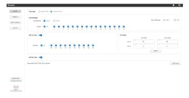
Custom scan is intended to be used when there is deeper investigation into specific lane-preset combinations needed or when a more comprehensive test of all lanes and presets is desired. Users can specify their own pass-fail limits and the Margin Tester will flag any results that fall outside these specified limits.
