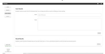
Results from any scan can be saved to a .zip file guickly and easily. All tabular data, like link training parameters and raw eye diagram measurements, are saved as .csv files and eye diagram images are saved as .png files.
