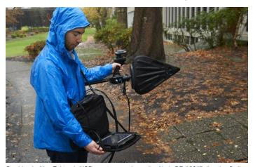
Combined with a Tektronix USB spectrum analyzer, the Alaris DF-A0047 direction finding antenna makes interference hunting easy. Lines of bearing are automatically transmitted from the antenna to SignalVu-PC Map software, enabling fast triangulation on interference sources.
