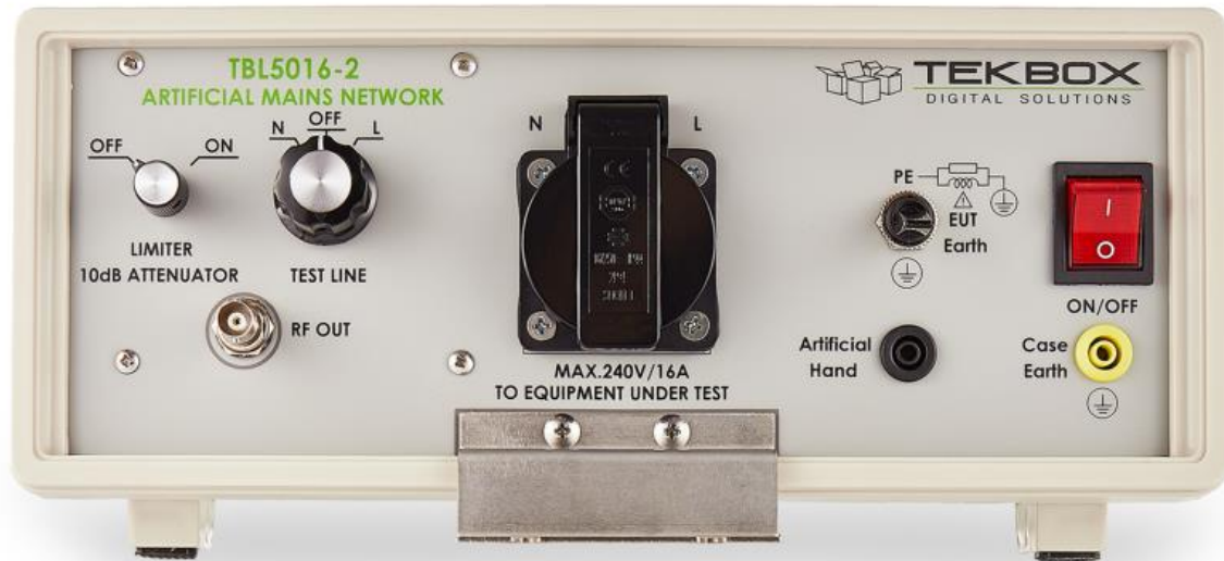
TBL5016-2 , variant with Schuko connector (CEE 7/3)
