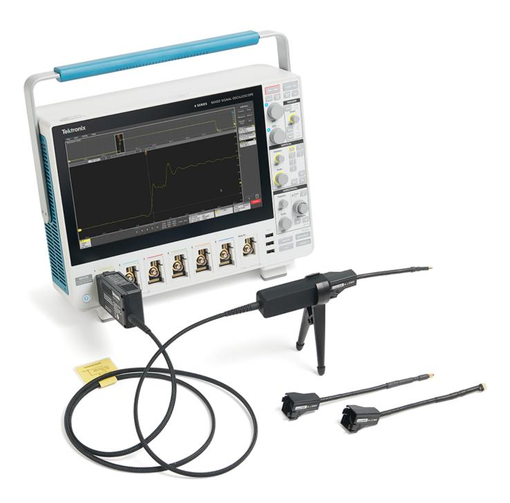
IsoVu probe technology delivers accurate differential measurements up to  $\pm 2500$  V on reference voltages slewing  $\pm 60$  kV at 100 V/ns or faster. With the IsoVu Generation 2 design, you get all the benefits of IsoVu technology at 1/5 of the size of first generation probes.
