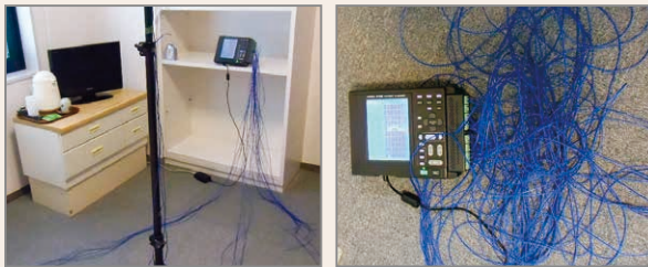
Long wires are used to connect the instrument to the measurement locations.
