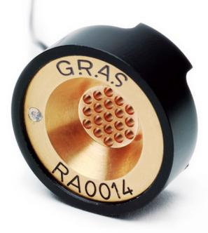
The GRAS RA0014 1/2" Electrostatic Actuator is an electrostatic actuator for testing the frequency response of standard 1/2", 1/4" and 1/8" microphones; adapters are included for testing 1/4" and 1/8"microphones. The GRAS RA0014 can be connected directly to the <u>GRAS 14AA Actuator Supply</u>.
