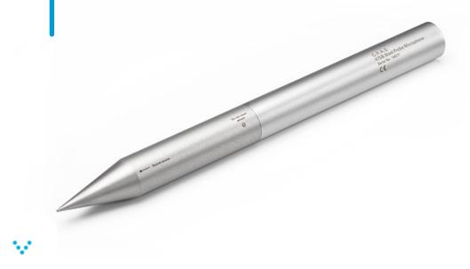
Freq range: 10 Hz to 20 kHz Dyn range: 52 dB(A) to 174 dB The GRAS 67SB Blast Probe is designed as a reference microphone for impulse measurements according to the ANSI/ASA S12.42 standard.
