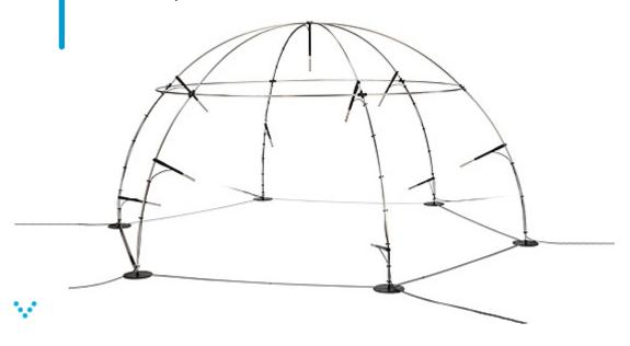
Freq range: 10 Hz to 16 kHz Dyn range: 6.5 dB(A) to 110 dB Sensitivity: 850 mV/Pa
