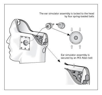
The transducers are mounted and removed by a simple snap-fit mechanism.
