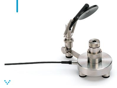
Connection: 200 V/LEMO Volume: 2 cc Dyn range: 25 dB(A) to 164 dB ANSI: S3.7 Type 2 IEC: 60318-5 The GRAS 43AB Artificial Ear is a complete test-jig for acoustical measurements on hearing aids.
