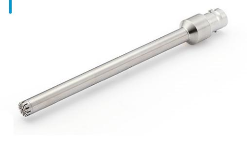
Freq range: 10 Hz to 20 kHz Dyn range: 32 dB(A) to 142 dB Sensitivity: 10 mV/Pa (± 3 dB) The GRAS 40PP-S1 QC Microphone, High Pressure is a robust, cost-effective microphone designed for use in production-line testing of loudspeakers and acoustic transducers. It has a wide frequency range reaching up to 20 kHz and a large dynamic range from <32 dB(A) to 142 dB.
