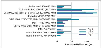
Figure 10. Spectrum Occupancy Measurement
