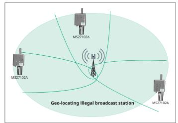
Figure 11. TDOA for Geo-Locating Interference Signal
