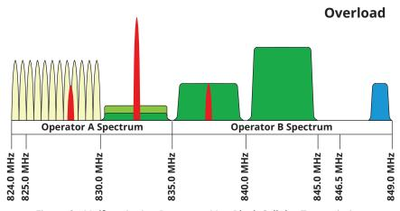
Figure 2. Malfunctioning Repeaters May Block Cellular Transmissions
