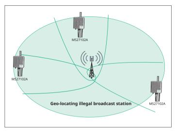
Figure 12. TDOA for Geo-Locating Interference Signal
