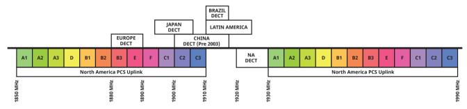
Figure 10. DECT Phones Improperly Used Can Cause Unintentional Interference
