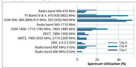
Figure 11. Spectrum Occupancy Measurement
