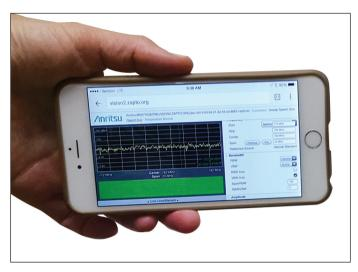
Figure 5. User Interface Displayed on Smartphone
