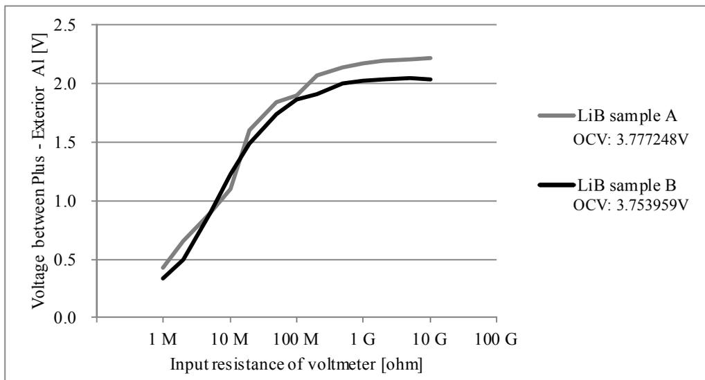
Fig. 5 Effect of package potential load resistance (voltmeter input resistance)
