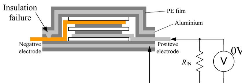
Fig. 11 Contact with a defect-free surface
