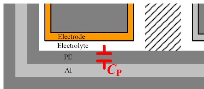
Fig. 9 Capacitance  $C_P$  between the package aluminum and electrodes
