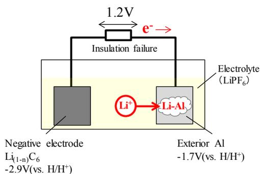
Fig. 2 Negative electrode insulation failure and cracking in package film
