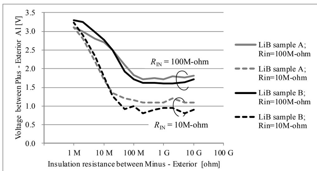
Fig. 8 Negative electrode insulation failures (simulated resistance) and package potentials
