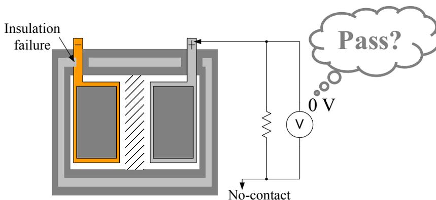
Fig. 10 Indication of 0 V due to a connection issue
