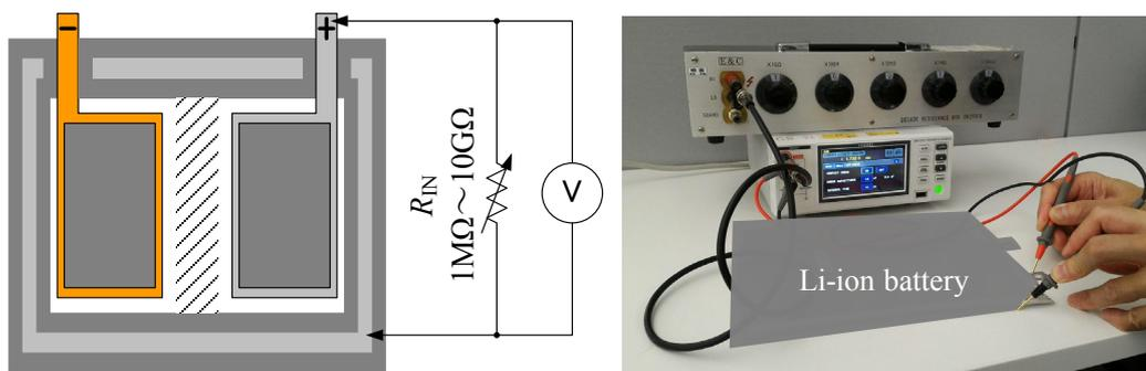
Fig. 4 Method for measuring package potential
