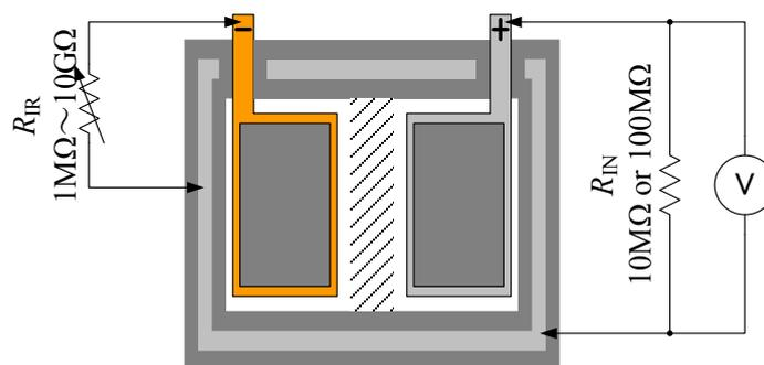
Fig. 7 Method for measuring package potential while simulating a negative electrode insulation failure
