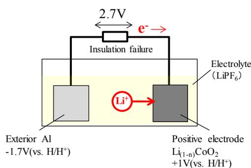
Fig. 3 Positive electrode insulation failure and cracking in package film
