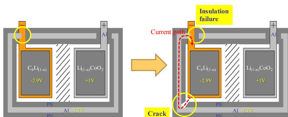
Fig. 1 Cracking in the insulating film
