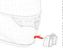
Carefully line up the mount with your helmet (remember step 1). Don't press untill you have the placement just right. When you think the mount is on the right spot, press hard and hold for at least 1 minute with firm pressure.
