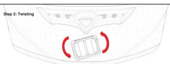
When the corners of the adhesive are released, try twisting the Go Moto mount (you can attach something to the mount to get more grip). For this step you can also heat op the mount a little more. By twisting the Go Moto mount it should release from your helmet. (Don't pull! This may damage your helmet!)
