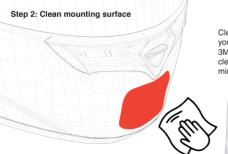
Clean the mounting surface on your helmet with the provided 3M VHB Surface Cleaner. After cleaning the surface, wait a minute to let it drv.
