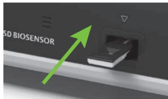
8. When inserting the test device to the analyzer, the analyzer will automatically scan and display the test results.
