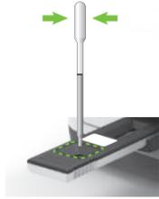
8. After applying the sample, immediately press the 'TEST START' button.
