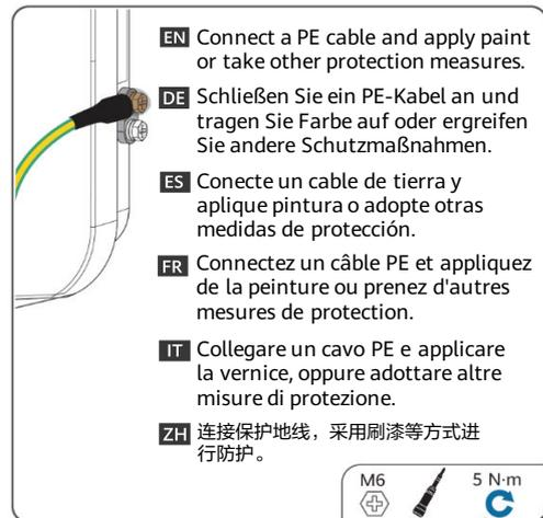
**EN** Connect a PE cable and apply paint or take other protection measures.
