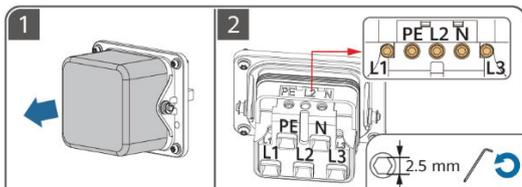
**EN** Connecting an AC Output Power Cable
