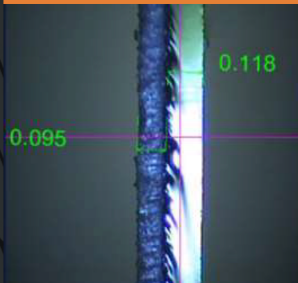
Rough surface resulting 80-120µm heat affected area
