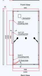
icon Sealan Laminate Laminate Frame 24.5 35 A-A B-B
