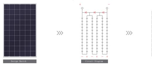
Module current output is 8.7A, current mismatch in series is **0.3A**.
