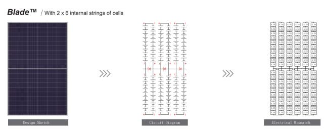
Module current output is 4.5+4.35=8.85A, current mismatch in series is **0.15A**.
