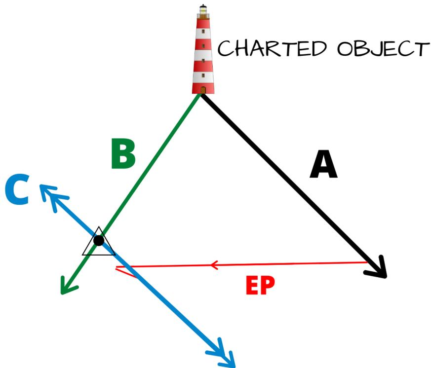
A running fix is a coastal navigation technique. It involves the use of an **estimated position (E.P)**. The fix is more accurate than an **E.P.** alone because it also incorporates bearings off of charted objects such as a lighthouse or recognisable headland.
