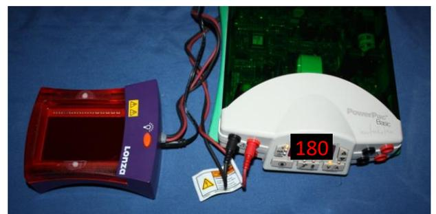
2.8 Watch progress of electrophoresis by switched on UV lamp of the dock.
