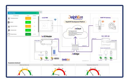
**D**elpheon is a digital twin monitoring application to analyse sensor data from buildings and operational installations. By collecting data from all kind of sensors (temp, electricity, gas, water, CO2, vibration, sound, laser optical, camera, read, ...) a digital twin portal is created to monitor the status of sensors, configure thresholds and alarms, sends notifications and make reports. Delpheon helps you saving time and money.
