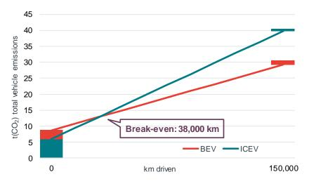
Figure 20. For LCVs with a small battery capacity, the breakeven point is achieved early on in the life cycle
