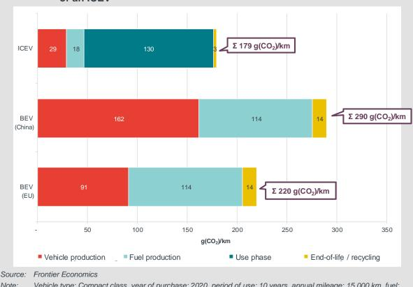
Figure 23. With the same range, almost as many emissions would be caused by the production of a battery for a compact BEV as over the entire lifetime of an ICEV
