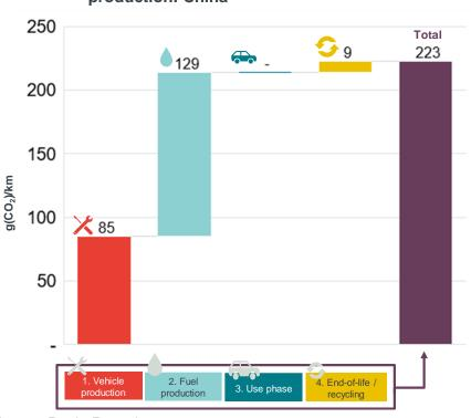
Figure 11. Overall CO<sub>2</sub> impact using the example of a medium-sized BEV – Country of battery production: China
