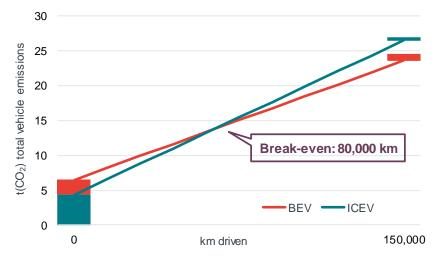
Figure 15. After 80,000 km, the emissions of the compact class BEV are lower than those of the ICEV
