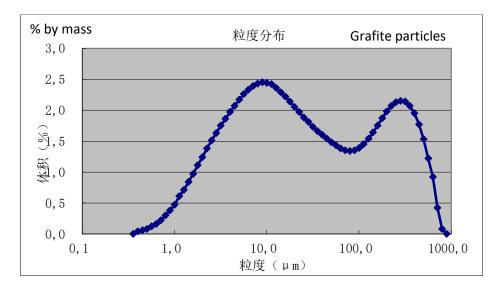
The distribution above is a favorable one and in a well-dimensioned cyclone we can expect to catch 99% of the particle-mass over 1 $\mu$ m and around half of the mass under 1  $\mu$ m.
