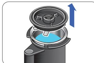
3. Remove the spray guard (8) and pacotizing blade (9) from the pacotizing beaker by pulling lightly on one of the three tabs on the spray guard.
