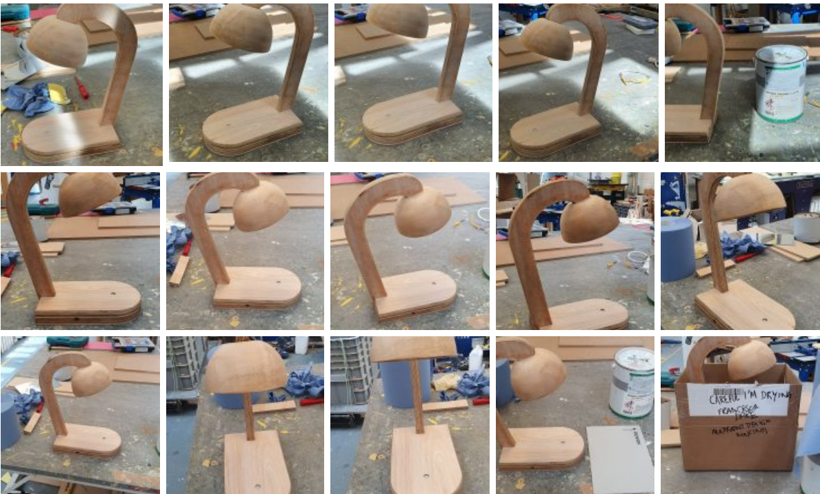
Finishing by sanding and applying multiple layers of wood wax.
